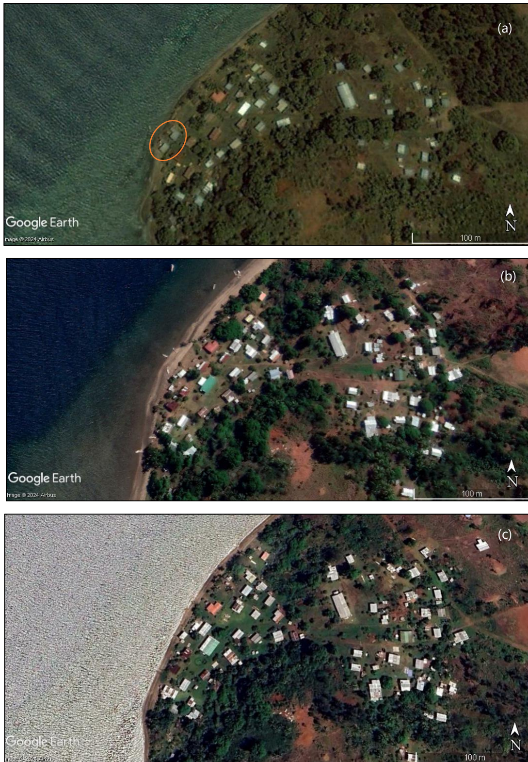
Figure 7.3 Historical Google Earth imagery has allowed a comparison of the foreshore of Naivaka from (a) October, 2008, (b) August, 2019, and (c) November, 2023 (Google, 2018). Loss of land can be noted, as well as houses in Figure 7.4 (a) that are not present in (b) and (c)
